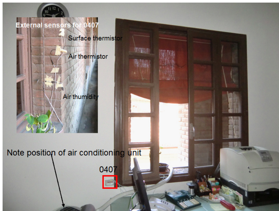
Figure 23: Positions of node 0407 with attached sensors.
