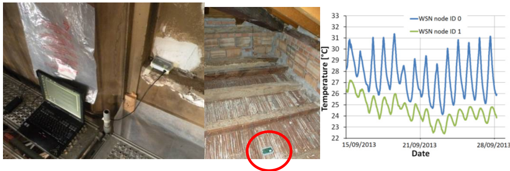
Figure 14: WSN monitoring of microclimatic conditions during refurbishment works: laptop and node 0 on the West wall of “Sala Urbana” (left), WSN node 1 in the roof space above the room (centre) example of monitor data (right), Source: [Colla C., Paci G., 2013], © DEI & DICAM Dept., University of Bologna
