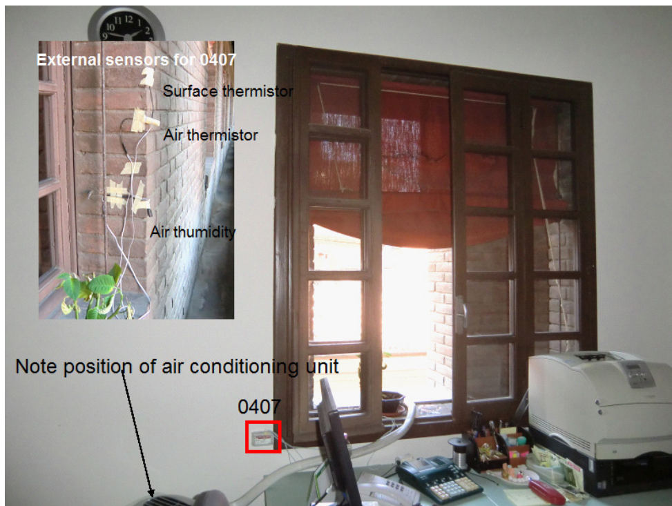
Positions of node 0407 with attached sensors.
