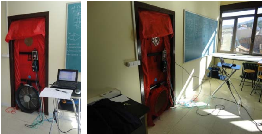
Figure 2: Blower door test in the physics laboratory
