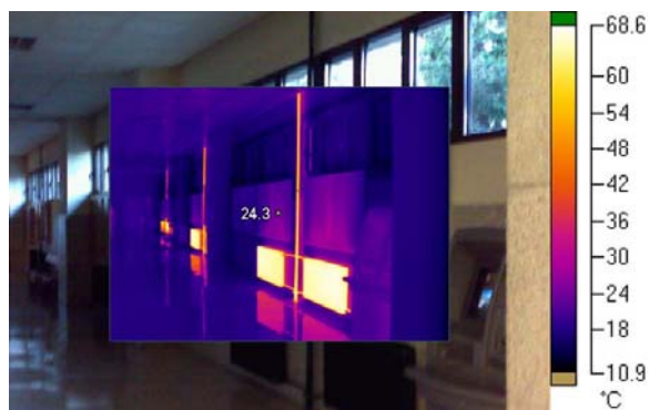
Figure 11: Radiators infrared thermography
