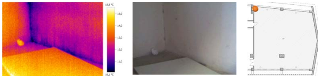
Figure 7: Junction thermal losses in the laboratory
