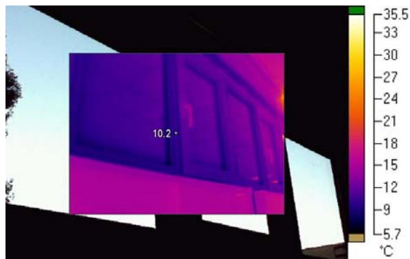
Figure 10: Windows infrared thermography
