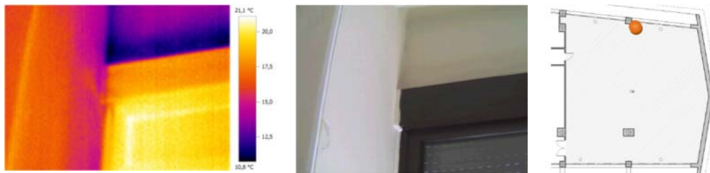
Figure 6: Blind thermal losses in the laboratory
