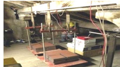
Wooden beam: load test
