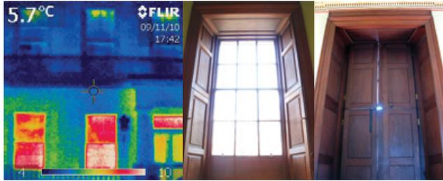
On the upper floor, the windows with the shutters closed show up in the thermal image in a deep blue colour, demonstrating how little heat is escaping.
