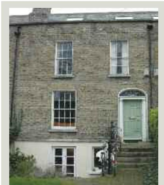
*The brick façade from 1821 was later repointed using a sand and cement mortar. While the removal of this pointing and its replacement with a vapour-permeable lime-based mortar would benefit the building, it is likely that the process of removal of the pointing would cause unacceptable damage to the brickwork*
