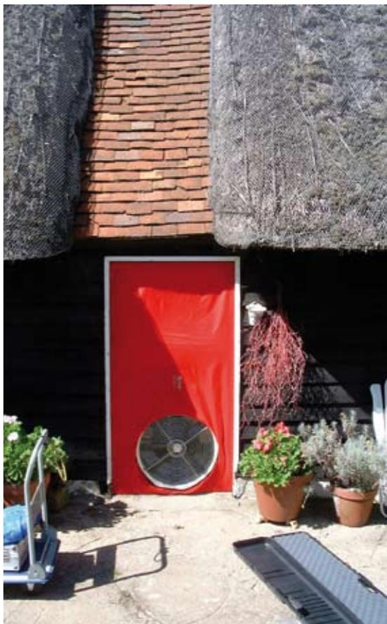
Pressure testing: fan equipment in operation at a doorway on the rear elevation
