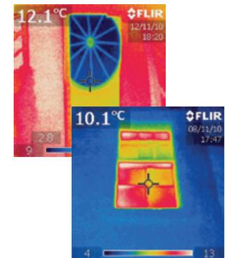
Heat loss: the Georgian cupola on the left is a cold spot, in blue in this interior thermal image; on the right, heat is escaping through a sash & case window, in red in this exterior image
