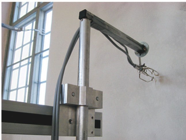
Figure 2 Ultrasonic anemometer mounted on a traversing device.
