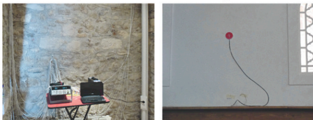
Figure 6. DAQ system at ground floor (left) and heat flux sensor on the upper floor (right)
