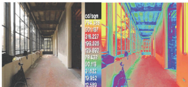
Figure 11 Visible image of the front loggia at the time of luminance survey (left), corresponding luminance distribution (right)
