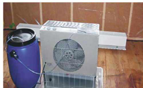
Figure 9 Example of a sensor arrangement for the monitoring in the construction element (above) and the controlling system for room heating and humidification (below).
