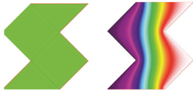
Figure 1 – Left: Sketch of double row honeycomb shades used for thermal calculation in THERM 7.1. Right: Temperature distribution of double row honeycomb shade determined by THERM 7.1.
