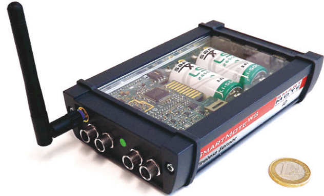
Figure 2 Wireless sensor node used for the impedance and temperature/humidity measurements.
