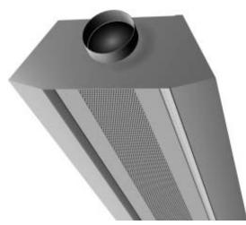
Chilled beams consist of water cooled finned tube convectors which make use of natural and/or induced convection to provide cooling. This is still a relatively new technology and only a small number of these systems have been installed.
