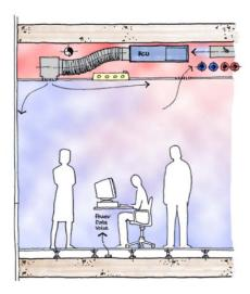
Fan coil unit ventilation systems are the most common form of air conditioning in many parts of the world. The popularity of FCU systems is due to the relatively low installation cost, flexibility of use, ability to deal with high heat loads, simple local control and reduced plant space.
