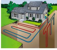
Shallow geothermal energy systems also known as ground energy systems, normally linked to a Ground Source Heat Pump (GSHP) are used as source of low CO2, low enthalpy energy to provide cooling and/or heating to buildings.
