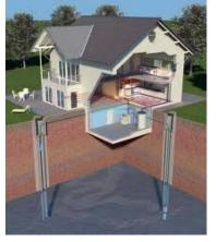
Open-loop use of ground water extracted from underground aquifers through boreholes, for cooling, or cooling and heating (using heat pumps). A typical borehole installation is hole with a steel pipe casing.
