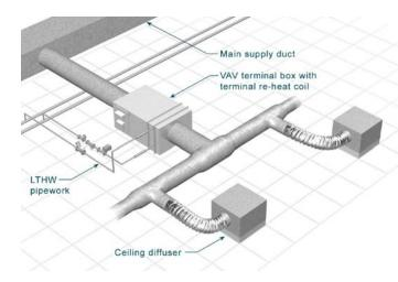
VAV is an all-air system with air supplied at a constant temperature with modulation of supply volumes to match the room sensible load. VAV is primarily to provide cooling and requires supplementary systems for heating
