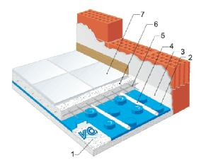
Underfloor heating UFH/Radiant floor works by passing low temperature hot water through pipework embedded in, or attached to, the floor. Heat is radiated from the floor and heats surfaces and objects in the room or space above.
