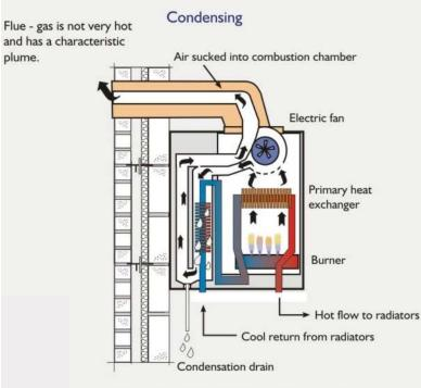
Combustion gases pass over primary heat exchanger and are then directed over secondary heat exchanger. As the gases condense on the sides of the exchanger they release their heat. Condensing boilers are composed by the same component of a traditional gas boiler. Their high efficiency is guaranteed by the energy recovered from the latent heat due by the condensation of the vapor contained in the combustion gases
