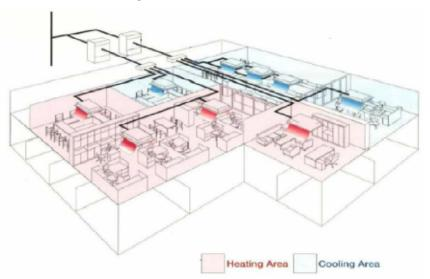
Variable refrigerant flow (VRF) systems, also known as variable refrigerant volume (VRV) systems, are essentially a multi-split DX system in which a number of indoor units are connected to a single outdoor unit.
