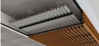
The chilled ceiling system is sometimes described as a static cooling system in that it transfers cooling to the room by natural convection and radiation in roughly equal proportions. It is a simple device that can offer an energy efficient solution in that distribution of cooling is principally by water and not air.
