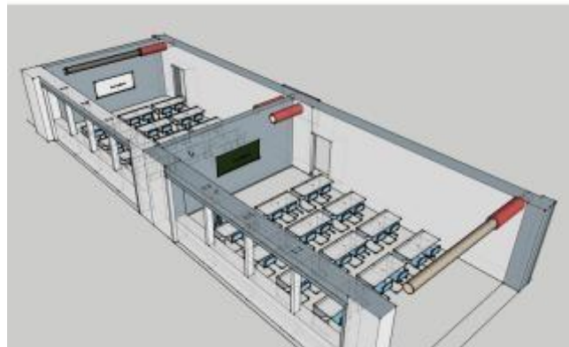
8: Monumental School, Innsbruck (Austria) – active overflow
