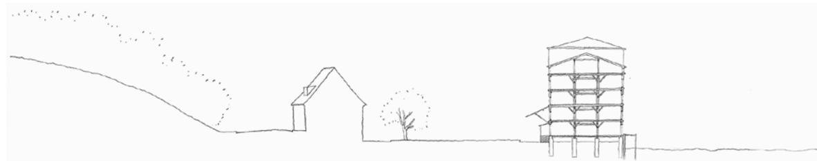
Figure 11. CS6, Schinkelspeicher, Potsdam; The section places the building on the waterfront, original to provide accessed to the Speicher/warehouse by boats. The building in between the hill and the water is a special climate condition. The original state of the building is a refined control of ventilation. Thus damage of humidity on the stored goods can be avoided. The building involves no thermal control.
