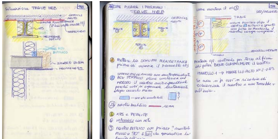
Figure 74: Documentation of 2 nd Workshop: Optimization of ceiling/wall connection (end of double-T-girder)
