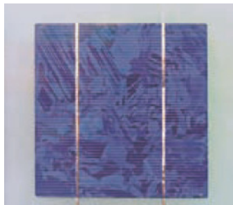
Figure 4: An individual polycrystalline silicon cell showing two busbars. Photo: Frank P. Palmer
