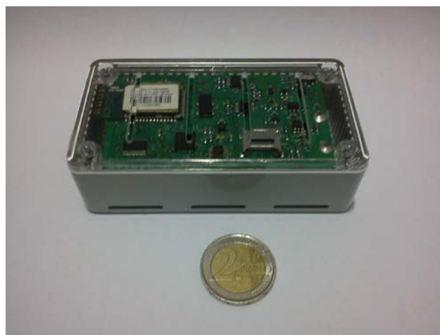
Fig. 2.2 Wispes W24TH inside the 98X54X29mm box
