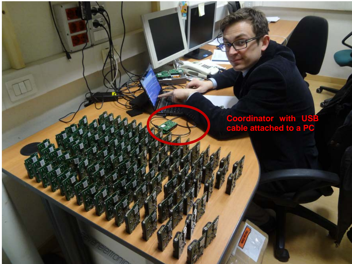
Fig. 9.1 3EncultWSN installation and test with 100 motes
