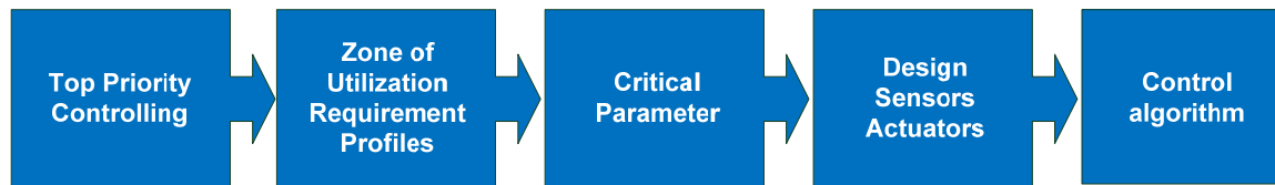
Figure 26: Development of a monitoring and control system in five steps
