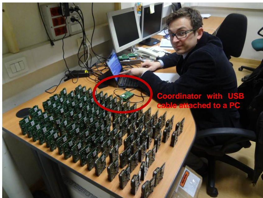
Figure 6: 3EncultWSN installation and test with 100 motes
