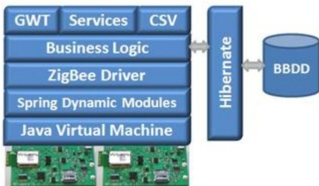
**A novel Building Management System (BMS) has been developed in the 3ENCULT Project which gathers monitoring information from a sensors network, known as "ZigBee", and displays the behaviour of the building in terms of the parameters measured. The system then calculates the best approach to take based on control algorithms.**
